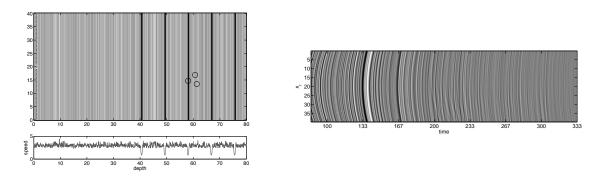
FIG. 2.3. Left: Simulation setup with a cluster of three scatterers buried in a layered structure with speed v(z) plotted below the computational domain. Right: Data traces plotted as a function of time (abscissa) and source-receiver offset (ordinate). The distances are scaled by the central wavelength and the time is scaled by the pulse width, which is 0.02s in our simulations.
