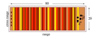
FIG. 5.1. Setup for numerical simulations with sources buried in a finely layered structure. The units are in carrier wavelengths  $\lambda_o$  and the distance d between the scatterers is 4. The perfectly matched layer surrounding the domain is shown in pink.
