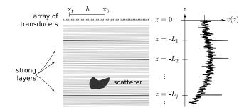
FIG. 1.1. Schematic of the setup for imaging scatterers buried in a layered medium with sound speed v(z). The array of transducers sits on top of the medium. The source and receiver locations are denoted by  $\mathbf{x}_s$  and  $\mathbf{x}_r$ . The medium is finely layered and it has some strong scattering interfaces at depths  $-L_j$ , for j = 1, 2, ...
