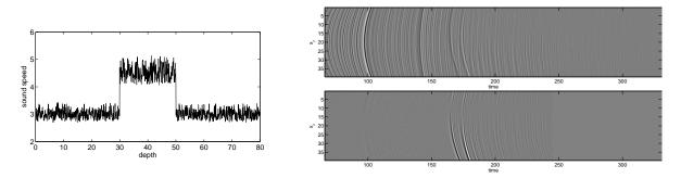
FIG. 5.9. Left: Sound speed v(z). Right: Traces before (top) and after (bottom) annihilation.
