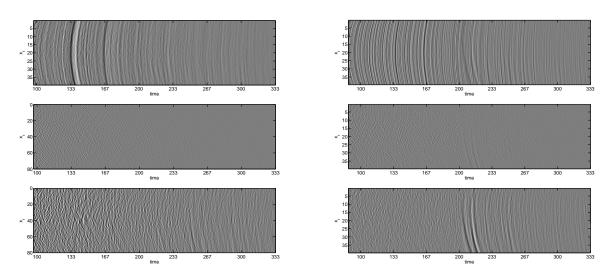
FIG. 5.11. Top: Raw traces for the layered structure plotted in Figure 2.3 and additional isotropic clutter. Middle: Traces filtered with the annihilator in Definition 3.1. Bottom: Traces filtered with the annihilator in Definition 3.3. Left: Isotropic clutter with 3% standard deviation. Right: Isotropic clutter with 1% standard deviation.
