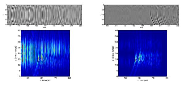
FIG. 5.8. Left: Traces and Kirchhoff migration image without annihilation. Right: Annihilated traces and the resulting migration image. The speed v(z) is as in Figure 5.7, but without the five strong scattering interfaces.
