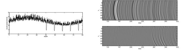
FIG. 5.7. Left: Sound speed v(z). Right: Traces before (top) and after (bottom) annihilation. The time axis is scaled by the pulse width and the receiver location is scaled by  $\lambda_o$ . The echoes from the small scatterers are overwhelmed by those from the layers in the top traces, but they are clearly emphasized after the annihilation.
