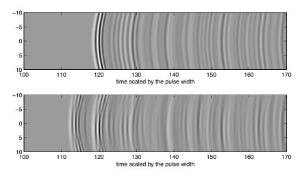
FIG. 5.2. Traces recorded at the array for a single source (top) and four sources (bottom). The pulse width is 0.02s.
