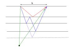
FIG. 3.1. Illustration of a primary path (red), a multiple path (blue) and a path through a point scatterer (green). At background speed  $c_o$  the multiple path maps exactly to a primary reflection at a ghost interface drawn with dotted line.
