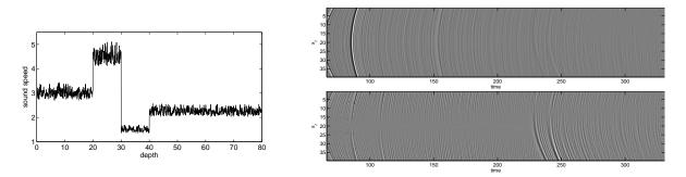
FIG. 5.10. Left: Sound speed v(z). Right: Traces before (top) and after (bottom) annihilation.
