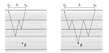
FIG. 2.1. Examples of coherent paths from the source at  $\vec{\mathbf{x}}_s$  to a receiver at  $\vec{\mathbf{x}}_r$ . Left: Path between the layers without "seeing" the scatterer at  $\vec{\mathbf{y}}$ . Right: Path through the scatterer at  $\vec{\mathbf{y}}$ .
