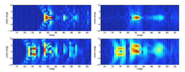
FIG. 5.3. Top: images with the traces in Figure 5.2 top for a single source. Bottom: images with the traces in Figure 5.2 bottom for four point sources. Left column: Kirchhoff migration. Right column: CINT. The correct location of the source is shown in each figure with a green dot.
