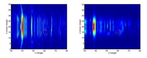
FIG. 5.4. Images with the traces in Figure 2.3. Kirchhoff migration is on the left and CINT on the right. The small scatterers are indicated with circles and they are invisible in both images. Both range and cross-range are scaled by  $\lambda_o$ .
