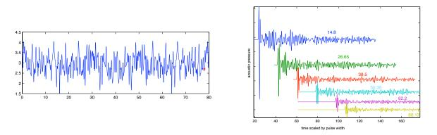
FIG. 2.2. Left: The sound speed v(z) as a function of depth measured in central wavelengths. Right: The transmitted pressure field for different depths traveled in the random medium. The depth for each trace is measured in central wavelengths.
