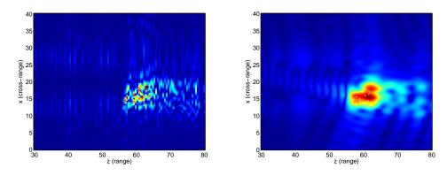
FIG. 5.5. Images with filtered data  $[\mathbb{Q}_{c_0}D](t,h)$ . Migration is on the left and CINT on the right.
