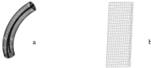
Fig. 2. Numerical grid of (a) the pipe bend and (b) cylindrical flat-bottomed bin
