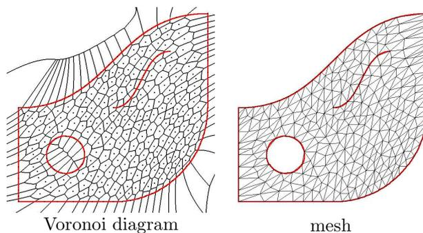
Figure 6: Input with straight lines, circles, and Bezier curves.
