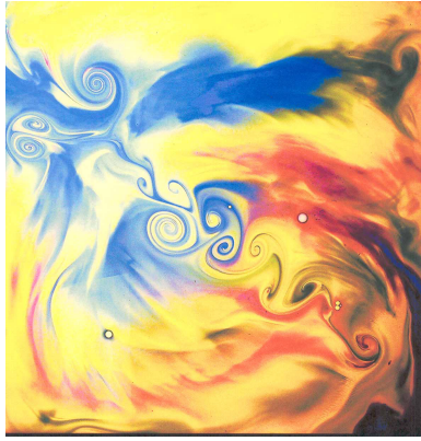
FIGURE 1. Photograph of vortices and vortex pairs which have been created by the motion of a particle on the surface of a fluid.
